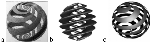
Figure 3: Trimming a spherical surface: a) "Sphere Spirals" (©2009 The M.C. Escher Company B.V., the Netherlands); b) a trimming solid; c) a trimmed sphere surface.
