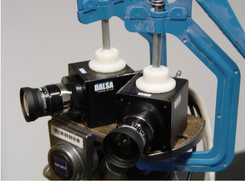
Figure 3: Camera setup: Two cameras fixed on a tripod, representing alignment in a circular camera array.
